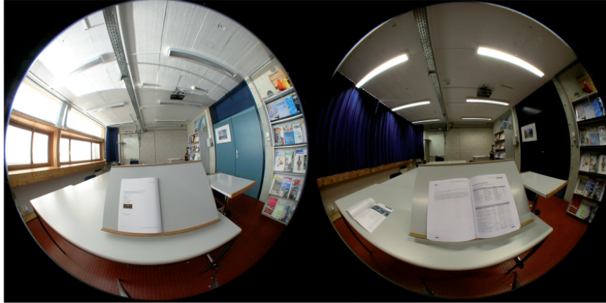
Figure 1 Photograph of the study room with the two different lighting conditions: (a) mainly daylighting conditions (DL); (b) electric lighting conditions (EL). The picture reproduces the view from the subject's position. The tilted board on the table ensured a more horizontal gaze direction
